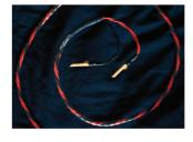
Normally used as a biwire cable, but wired on test as a single pair, this twisted-quad, single strand cable with FEP (fluorinated ethylene propylene) insulation looks plain
